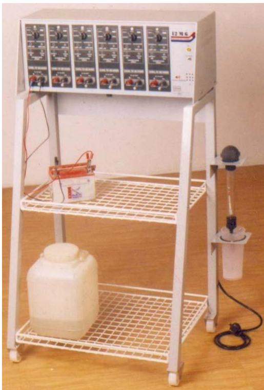
Battery Charging Station ( BCS 3)
